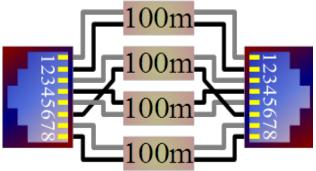
GAJ Technology's wireline simulator reproduce the characteristics of 4 pairs (8-wire) of CAT6 network cable with an RJ-45 connector at each end. The simulator can test any devices that use network cables such as routers, DSLAM, etc.
